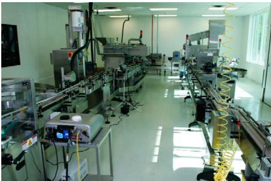
To maximize production throughput in a tight space, the supplier designed the new line in the shape of a key hole.
