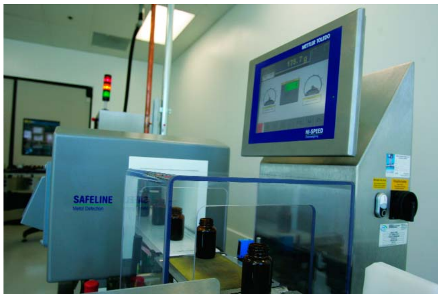
The checkweigher-metal detector verifies fill weight and accurately detects contaminants thanks to circuitry that counters electromagnetic interference from nearby process equipment.
