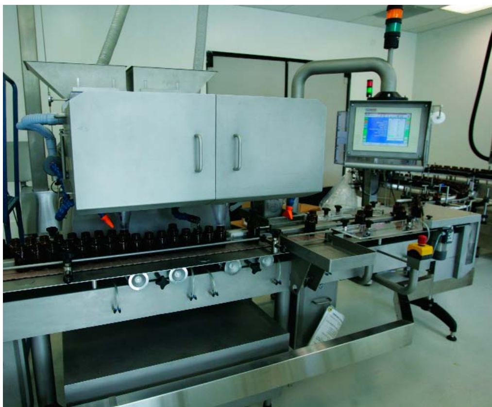
Metagenics' new line is anchored by a double-head tablet counter, which boosts capacity without increasing changeover time.
