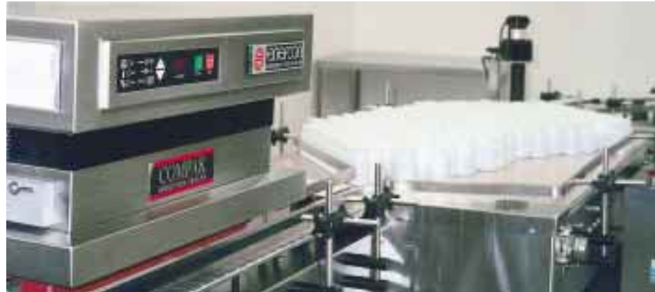
During counter operation, tablets are fed from 12 vibrating channels (per filling head), above, into a chute, where light beams register the size and shape of each tablet. Below, capped bottles are induction-sealed and then gather on an accumulation table to await labeling.
