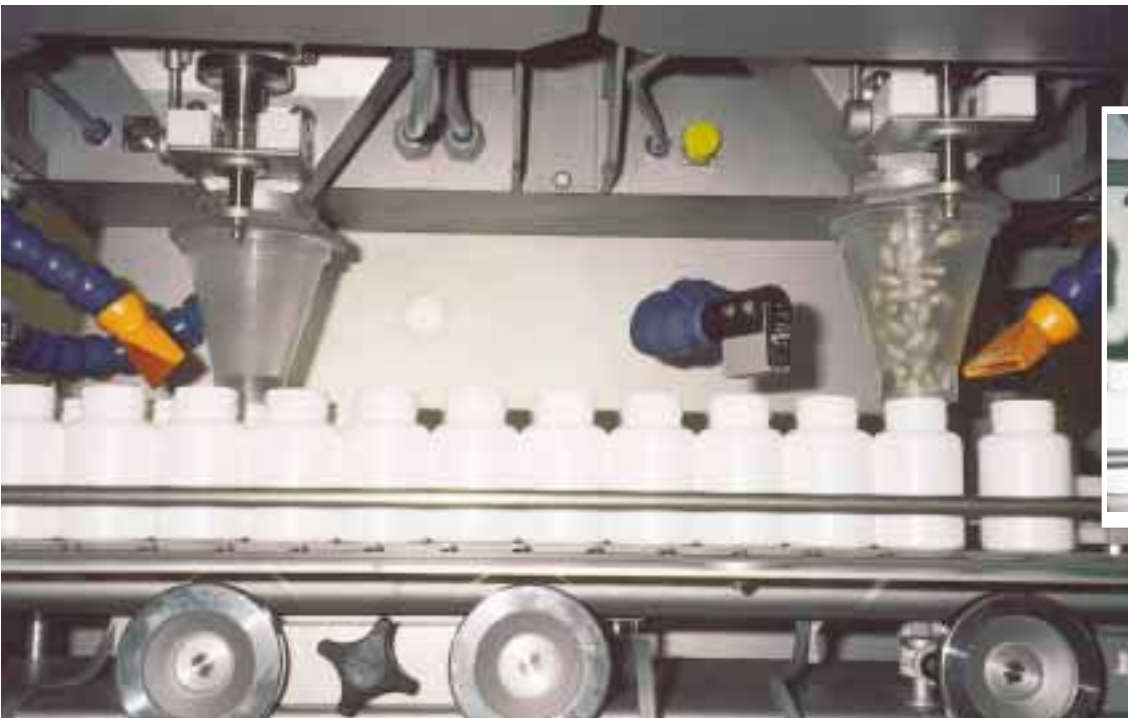
J.B. Laboratories chose a dual-head electronic counter, below, to fill a range of 10 PE bottle sizes with nutritional supplement tablets in a variety of shapes, due to the counter's changeover flexibility.
