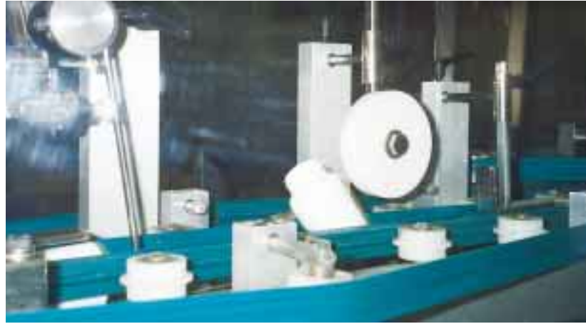
Bottles are manually dumped into the hopper from a plastic-lined shipper and enter the belt-style unscrambler, where they are inverted, cleaned with an ionized air rinser, and then uprighted.
