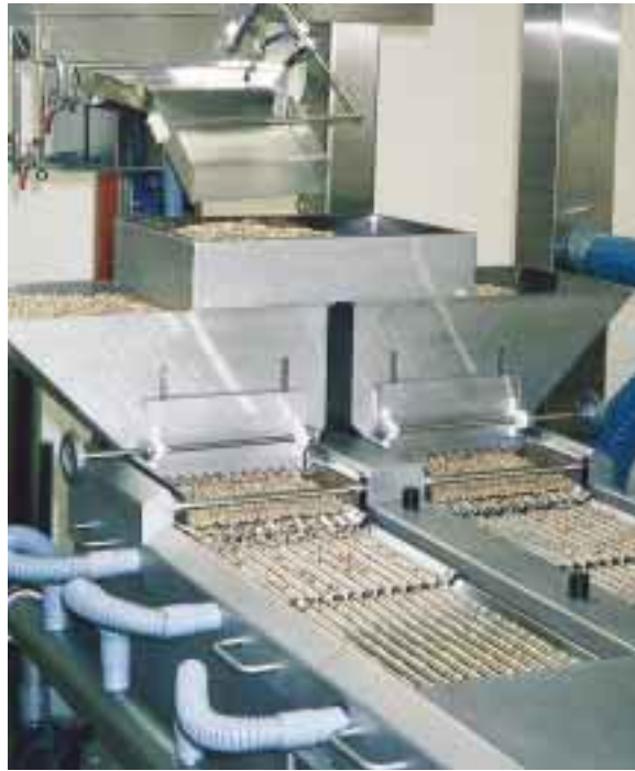
During counter operation, tablets are fed from 12 vibrating channels (per filling head), above, into a chute, where light beams register the size and shape of each tablet. Below, capped bottles are induction-sealed and then gather on an accumulation table to await labeling.
