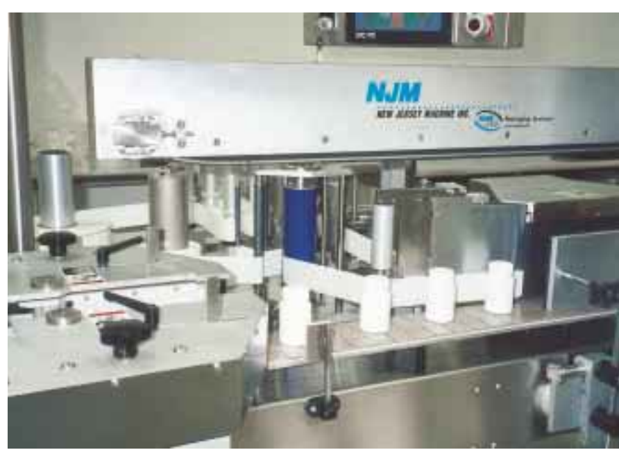
A p-s label applicator applies wraparound labels to the bottles after matching each label to the product being run by scanning a preprinted bar code on the label.
