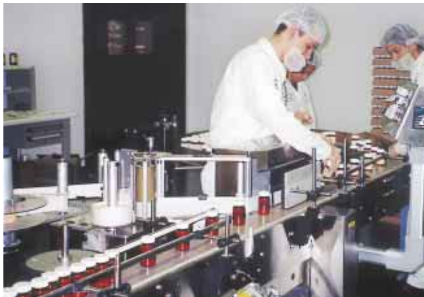
Following application of wraparound p-s labels, two operators inspect and pack off the completed packages into trays for insertion into master shippers.
